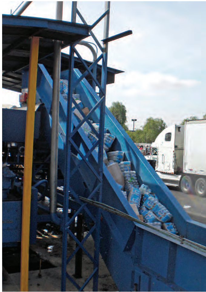
Conveyor feeding into a shredder
