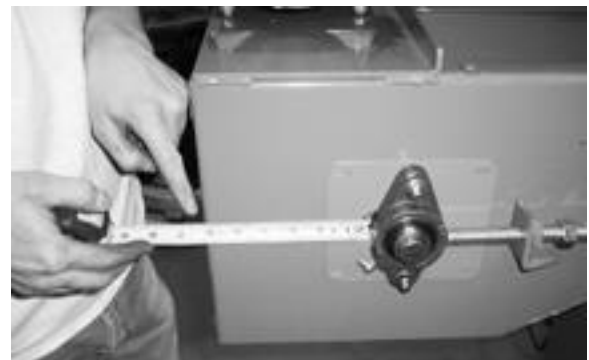
Figure 6. Checking for Headshaft Skew
