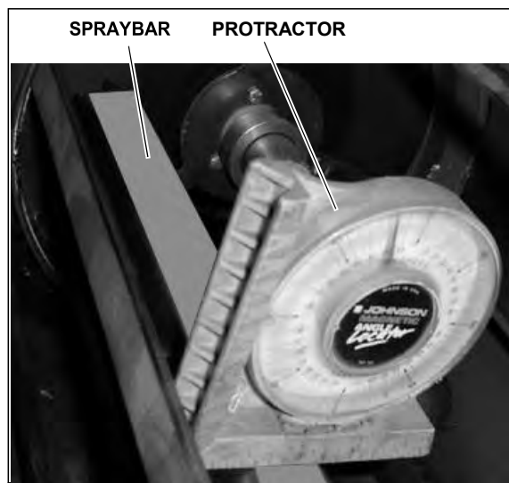
Figure 31. Setting the Spraybar Angle Using a Magnetic Base Protractor
