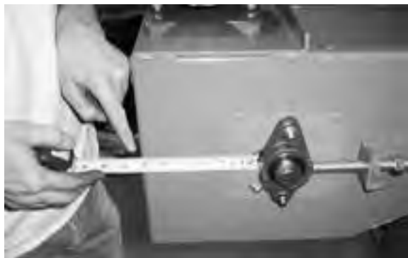
Figure 7. Checking for Headshaft Skew
