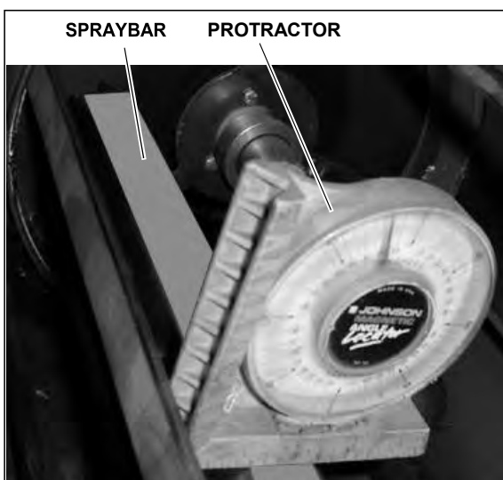
Figure 19. Setting the Spraybar Angle Using a Magnetic Base Protractor
