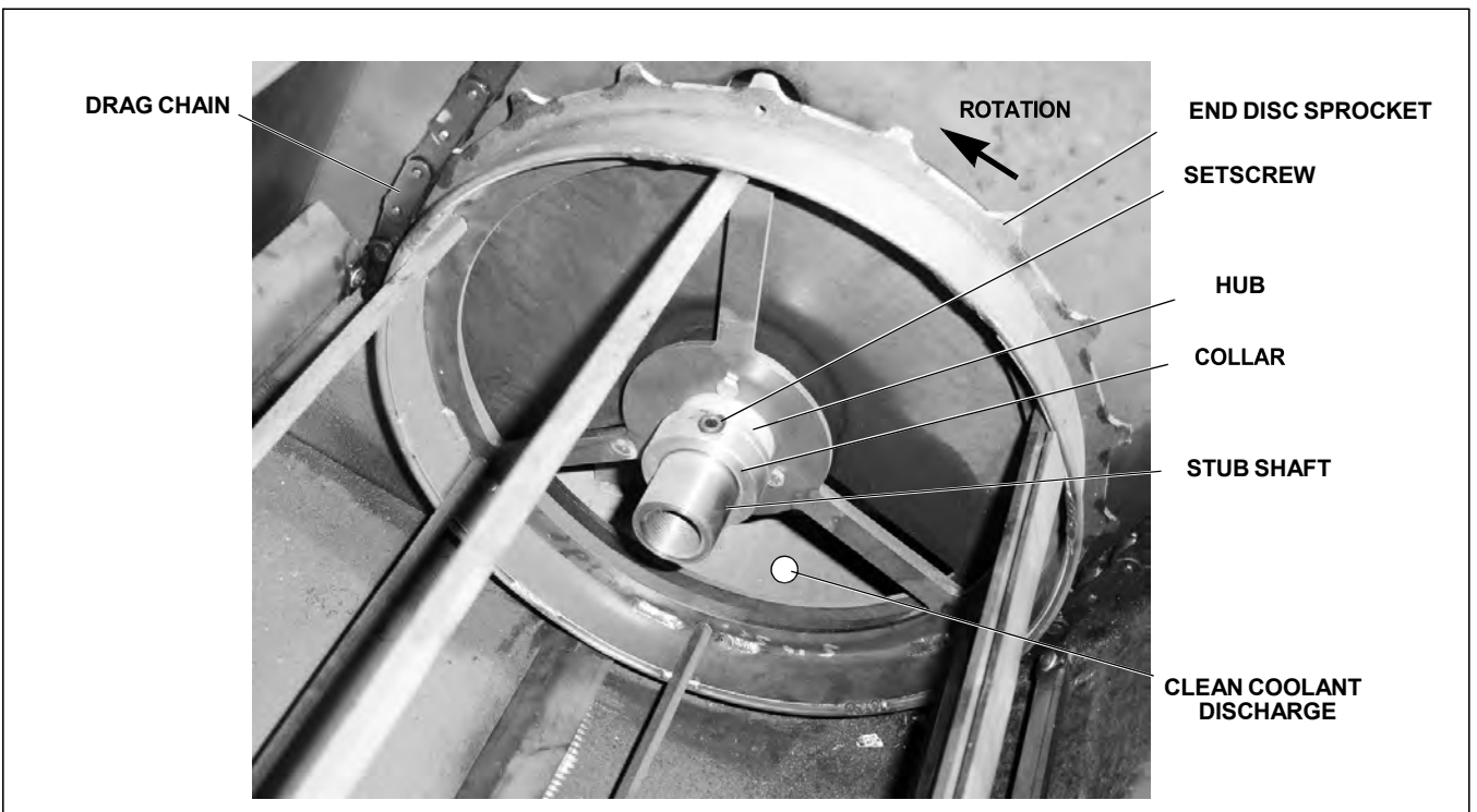
Figure 12. End Disc Assembly
