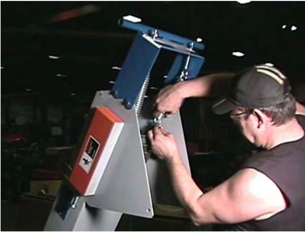
Unhook lanyard cables from ends of springs and remove.
