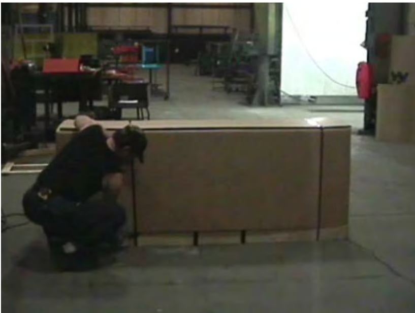
Remove banding from the corrugated cover on skid.
