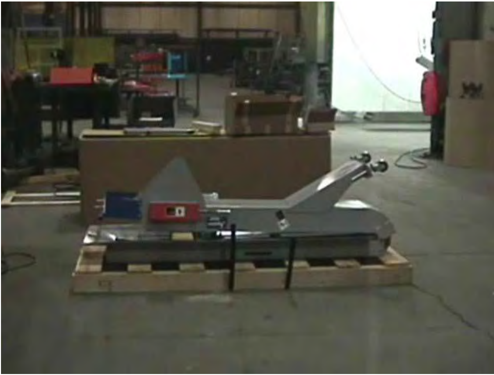
Conveyor after banding is cut, loose parts removed, and casters installed.
