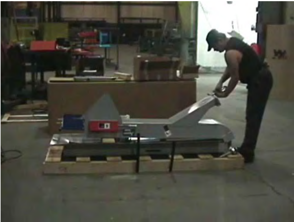
Screw casters into leg of conveyor.
