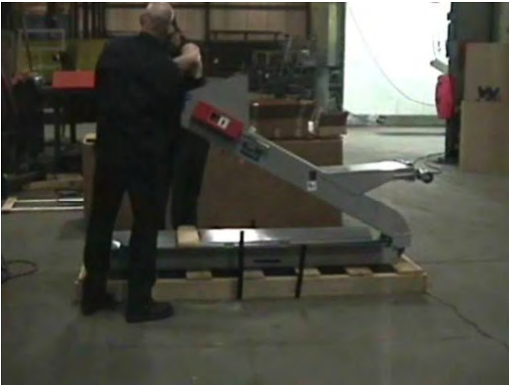
Unfold conveyor, we recommend that two people perform this task.
