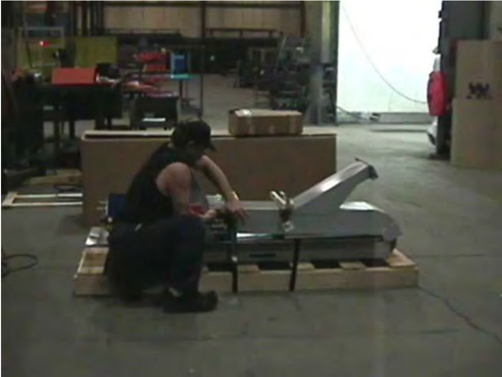
Remove banding from conveyor.
