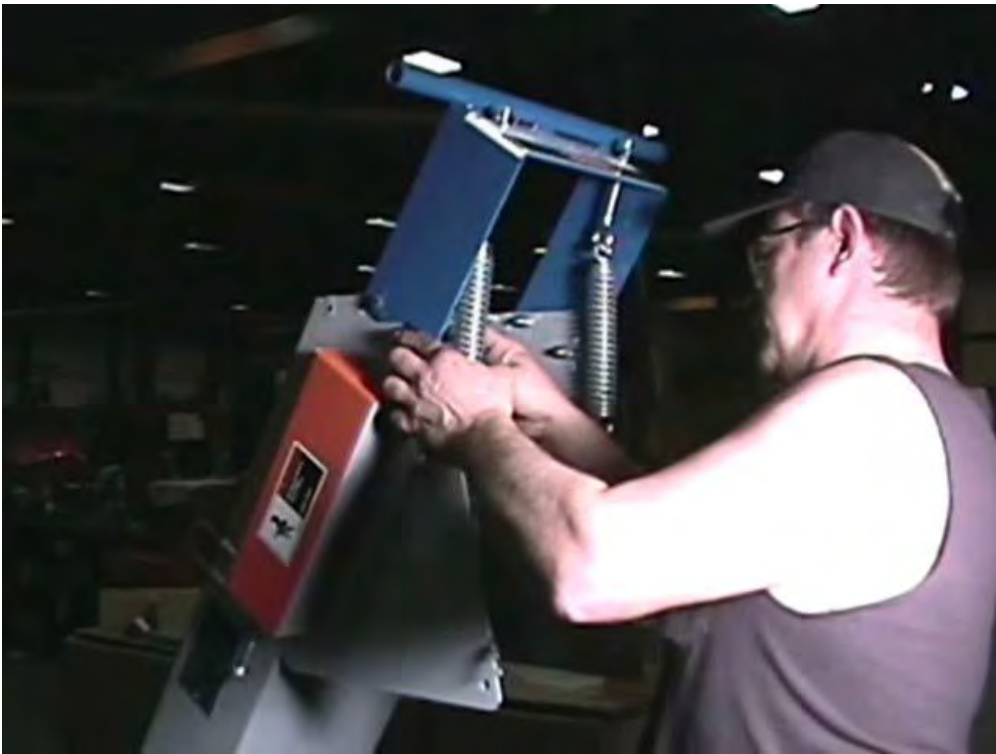
Using specified tools (see list in back) remove spring tensioning bracket from conveyor.
