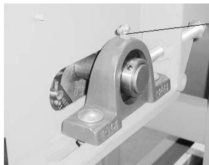
Figure 23: Grease fitting location
