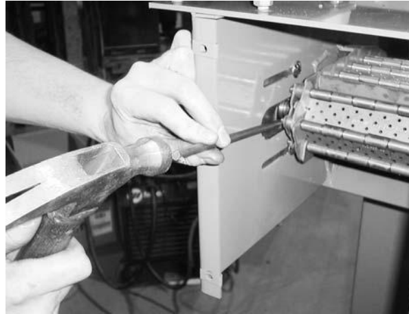
Figure 22: Installing the axle pin in the drive side
