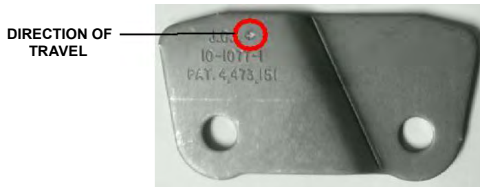
Figure 20: Belt direction indicator
