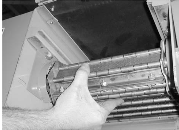
Figure 13: Checking Metal Belt Tension
