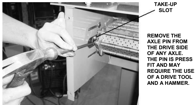
Figure 14: Removing the axle pin
