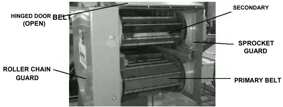
Figure 1: Discharge end of the conveyor
