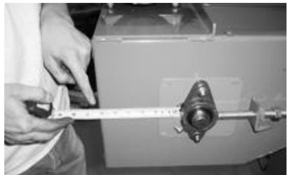
Figure 6. Checking for Headshaft Skew
