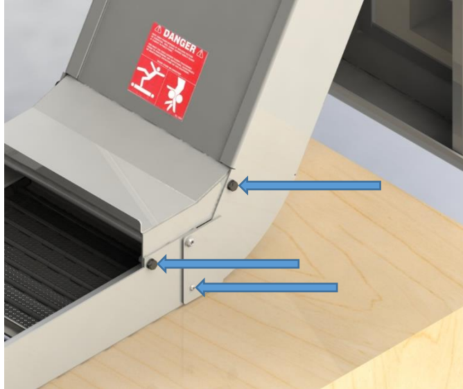
Figure 1.6 – Lower Curve Suppressor & Fasteners Installed
