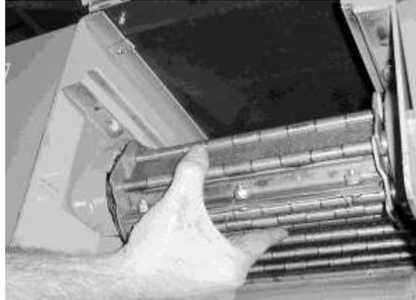
**Figure 14: Checking Metal Belt Tension**
