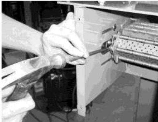
**Figure 15: Removing the Axle Pin**
