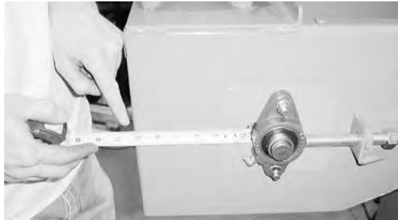
Figure 6 - Checking for Headshaft Skew
