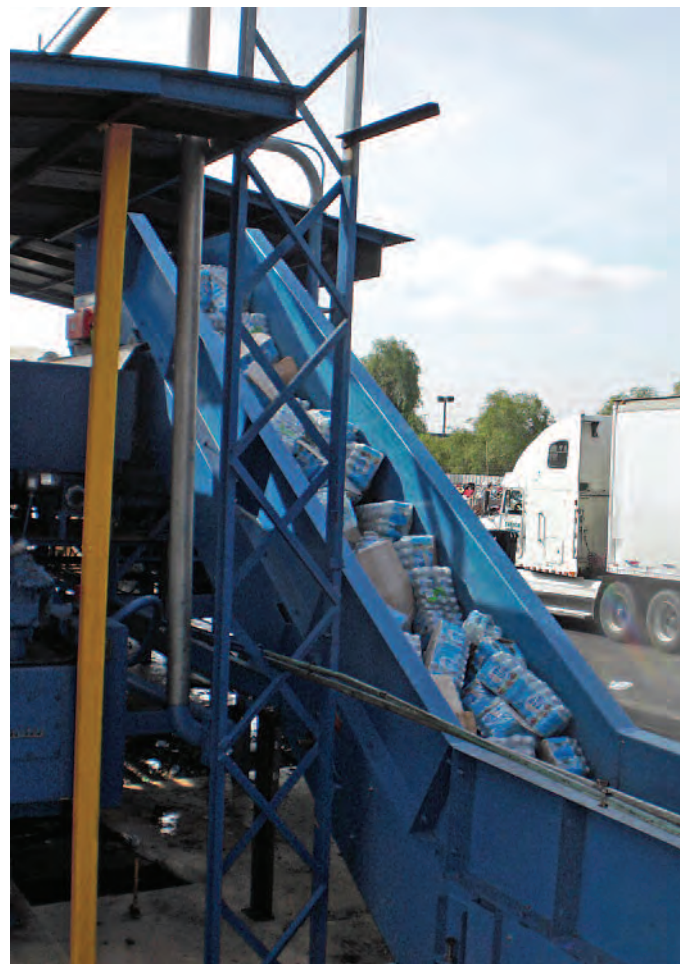
Conveyor feeding into a shredder
