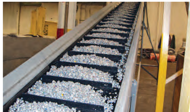
Cleated Transfer Conveyor moving paper pellets
