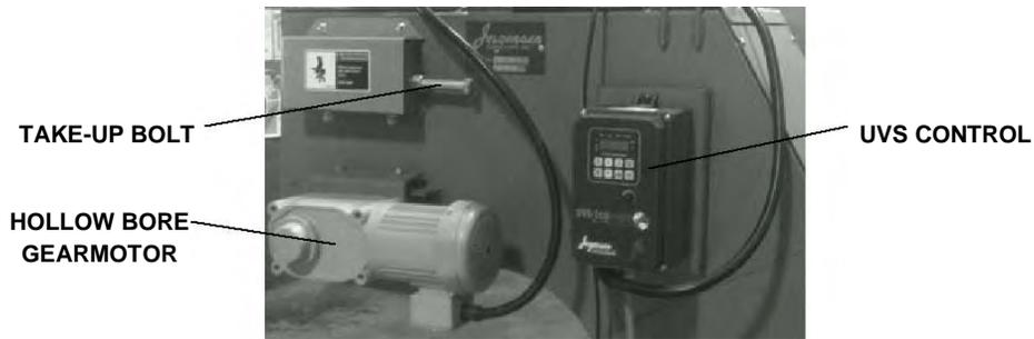
**Figure 5: Direct drive side of conveyor**
