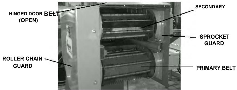
**Figure 1: Discharge end of the conveyor**
