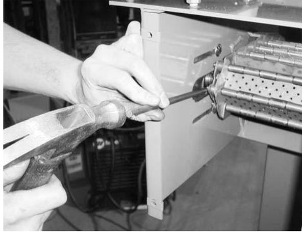
THE AXLE PIN IS PRESS FIT IN THE AXLE. INSTALL THE AXLE PIN IN THE DRIVE SIDE USING A DRIVING ROD AND HAMMER.
