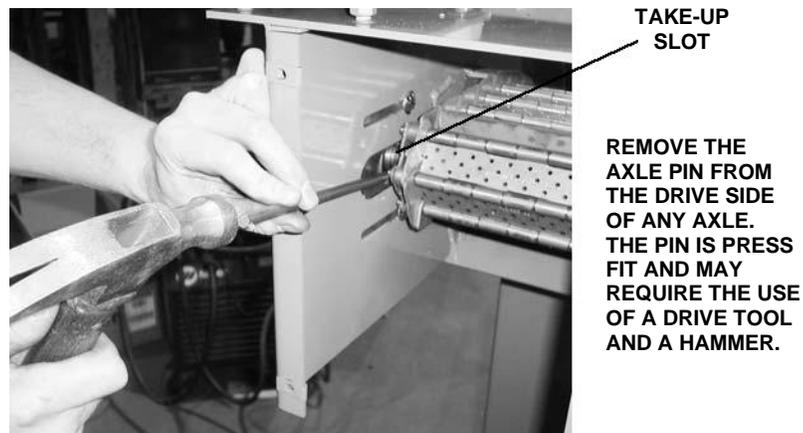
**Figure 14: Removing the axle pin**
