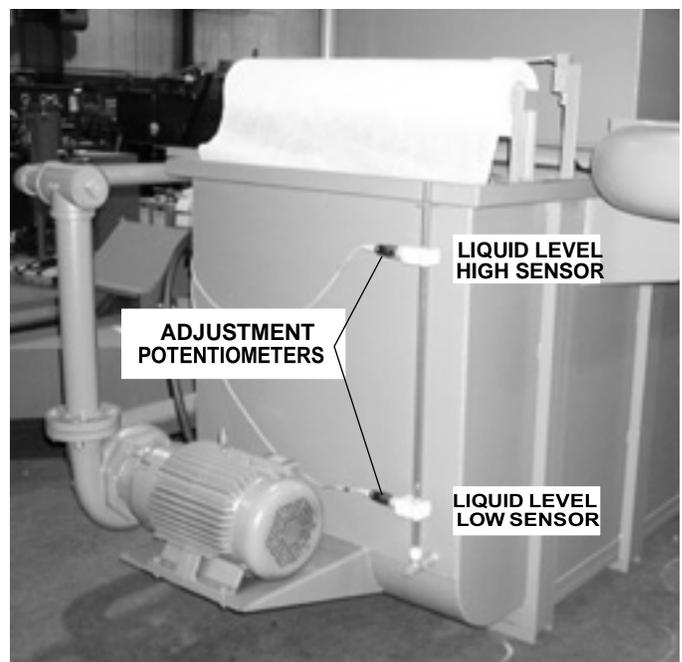
Figure 4. High and Low Liquid Level Sensors
