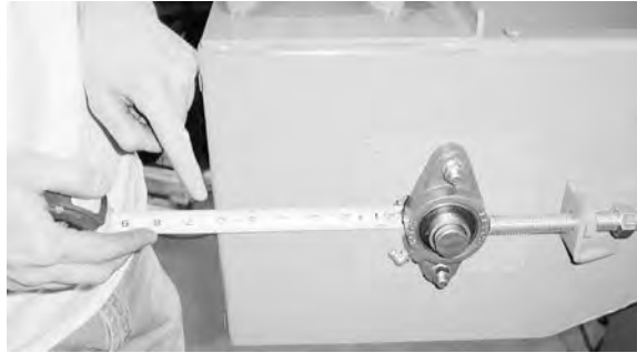
Figure 11: Checking for Headshaft Skew
