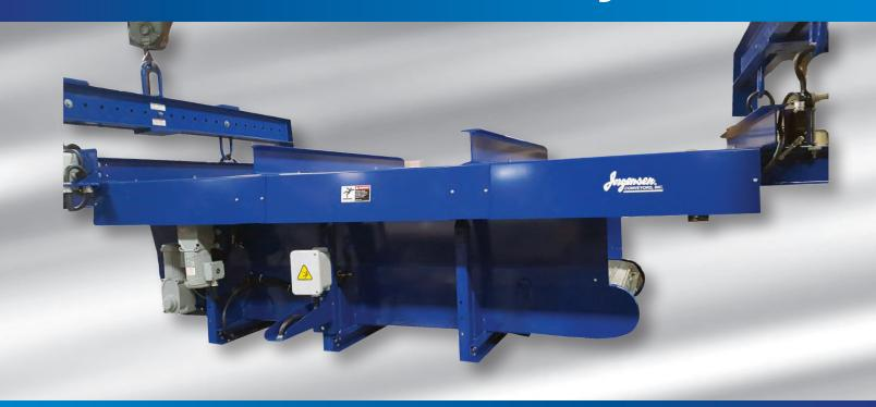
The new ShuttlePro® conveyor system is the ideal solution for automated level loading of chips into large in-plant central collection roll-off containers or truck trailers.
