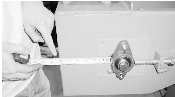
Figure 6 - Checking for Headshaft Skew
