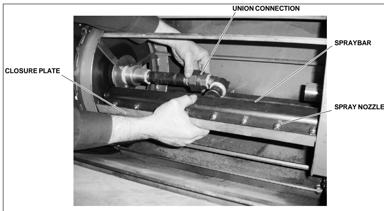
Figure 17. Disconnecting the Union Connection
