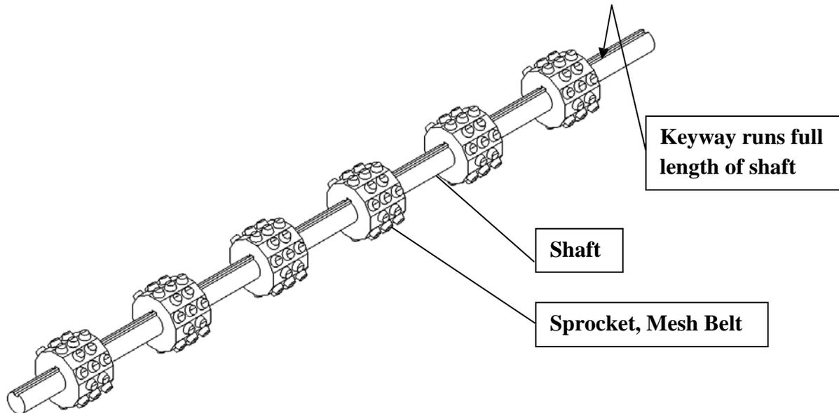
Fig. 3-8 Drive Shaft w/o Drive Sprocket and Bearings
