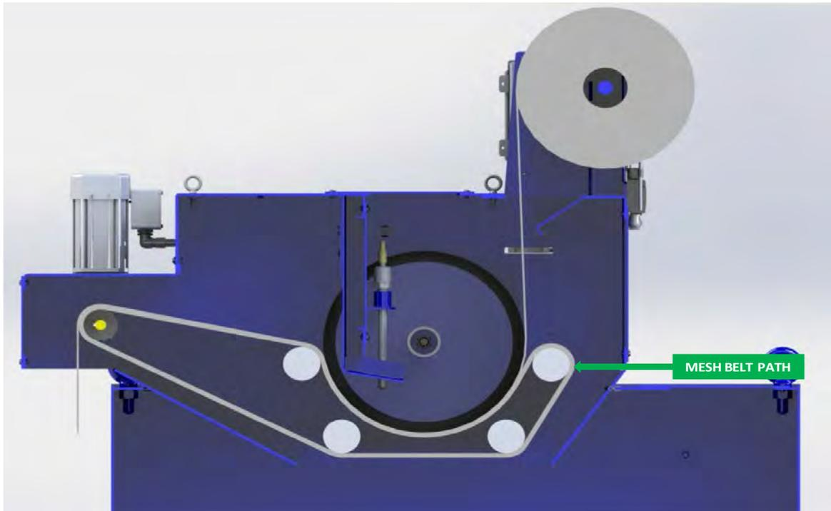
Fig. 3-9 Path of Mesh Belt through Filter
