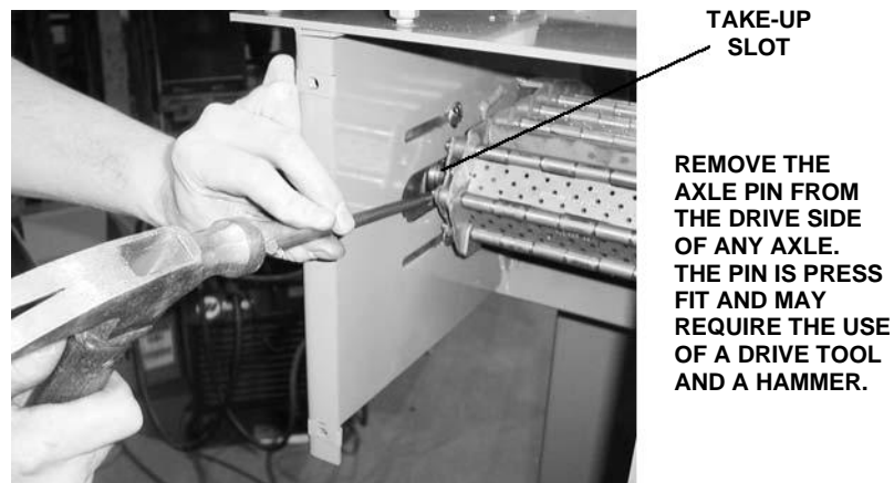
Figure 14: Removing the axle pin
