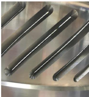
Slots machined into steel bowl
