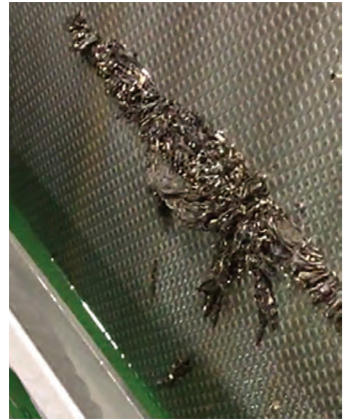
Ferrous chips being pulled up the incline section of the conveyor unit
