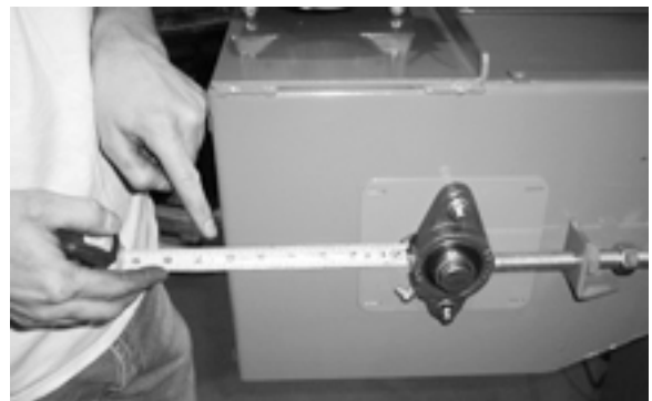
Figure 6. Checking for Headshaft Skew
