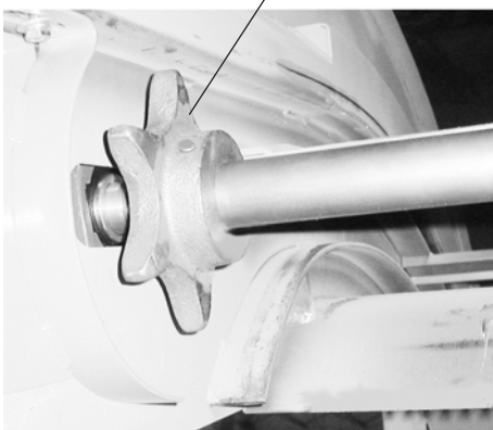
Figure 14. Removing the Sprocket Pin
