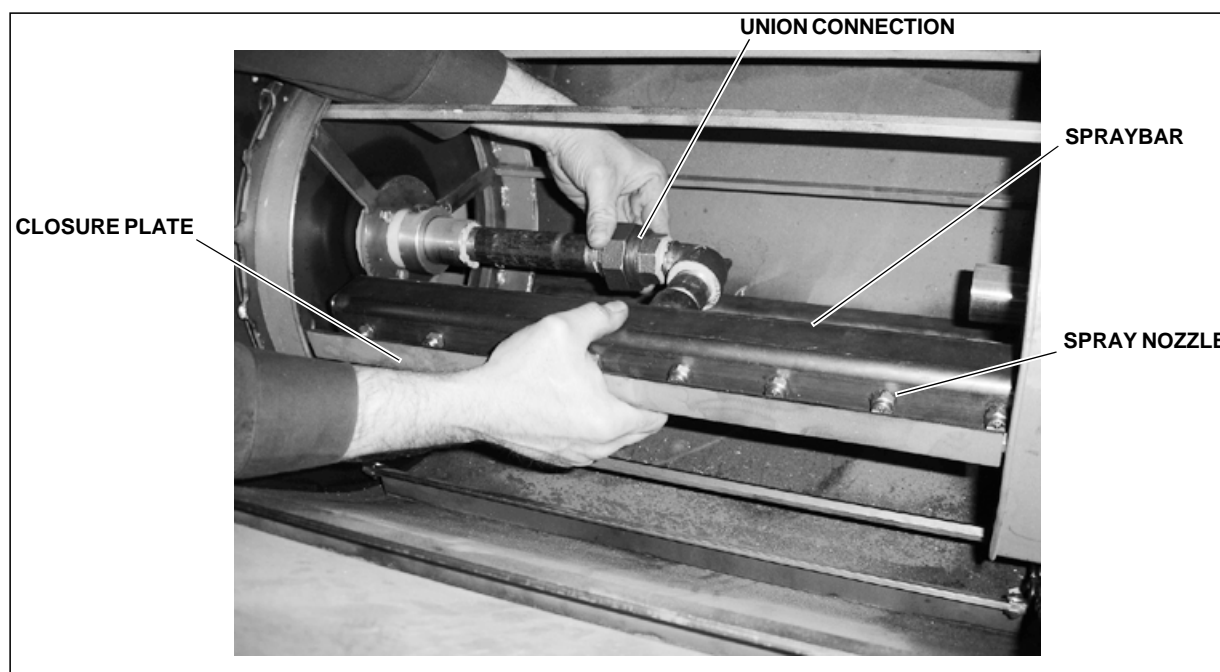
Figure 28. Disconnecting the Union Connection
