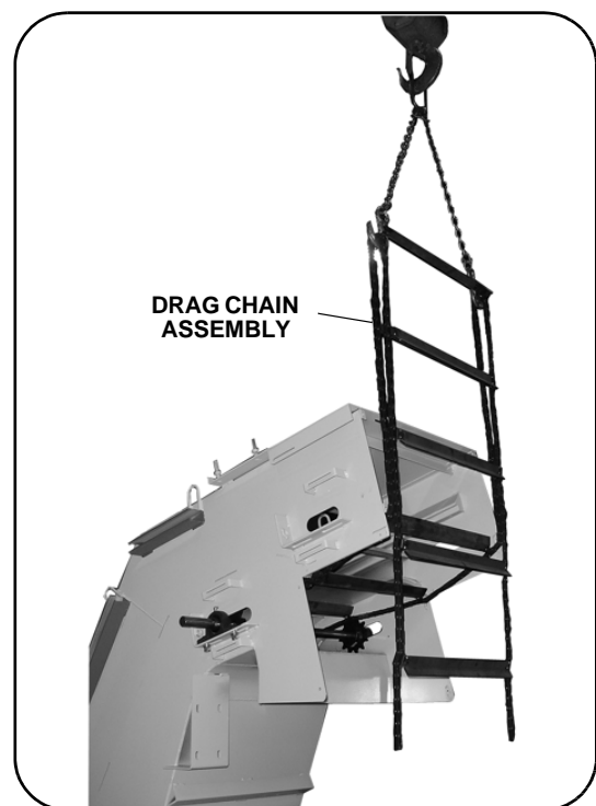
Figure 20. Removing the Drag Chain
