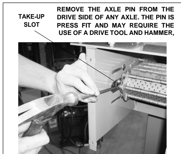
Figure 13. Removing the Axle Pin
