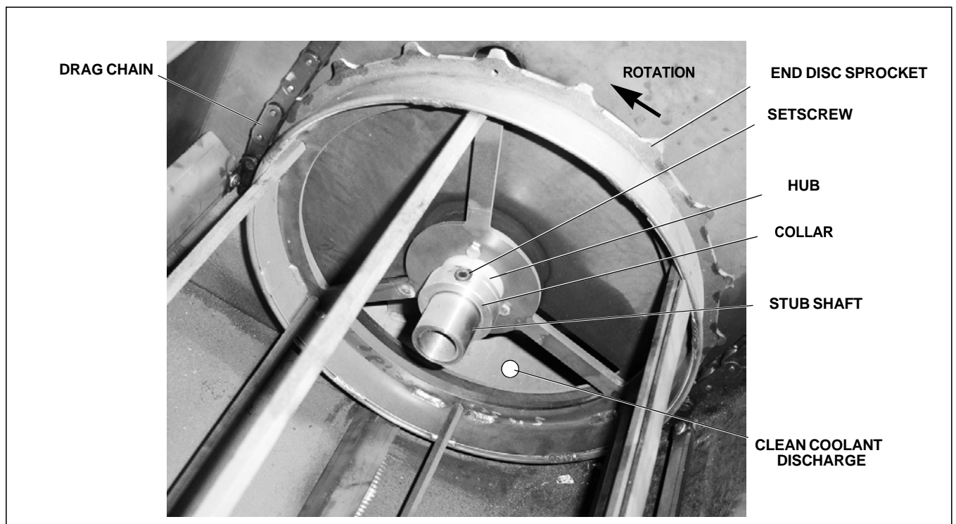
Figure 12. End Disc Assembly
