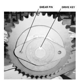
Figure 13: Driven Sprocket Shear Pin and Drive Key
