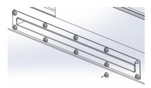
Figure 19: Remove fasteners
