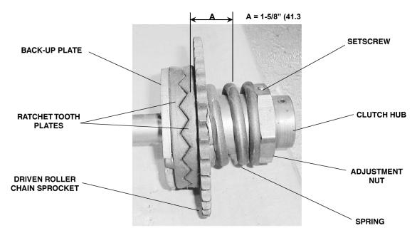
Figure 8: Ratchet Slip Clutch
