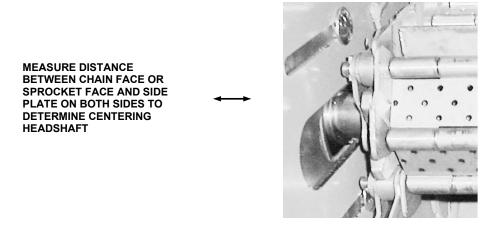
Figure 9: Headshaft Centering Measurement
