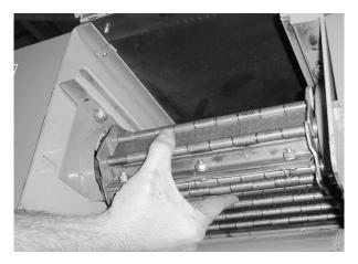
Figure 14: Checking Metal Belt Tension
