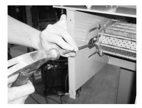
Figure 15: Removing the Axle Pin
