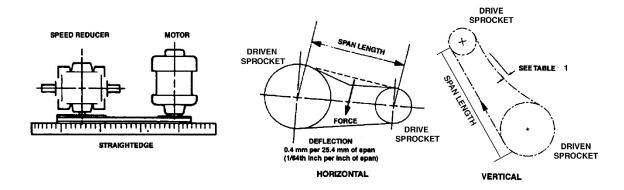
Figure 7: Reducer/Motor Alignment and Tension Adjustment
