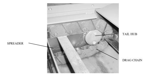
Figure 5: Tail end of drag chain conveyor.
