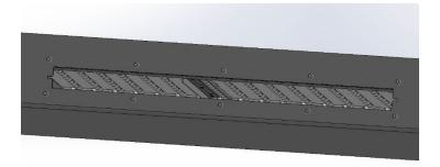
Figure 27: Brush in Inspection Window
