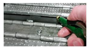
Figure 25: Spray Thru Openings
