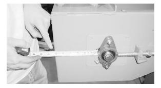
Figure 11: Checking for Headshaft Skew
