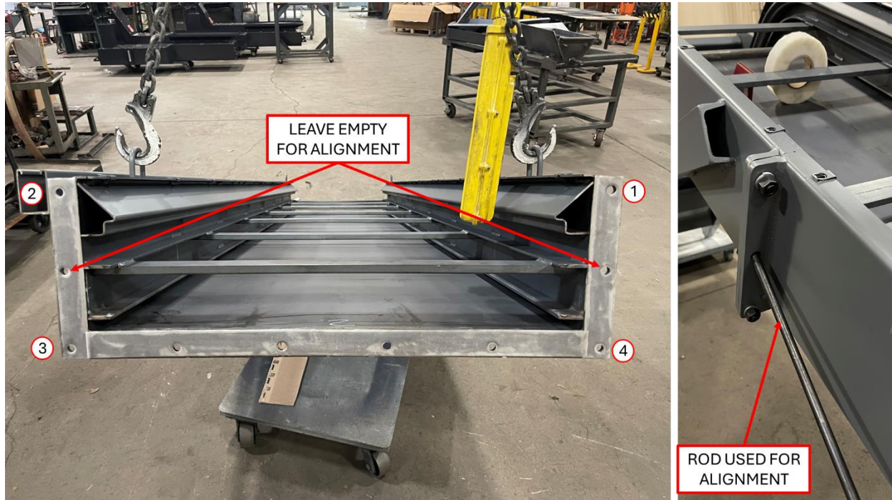
Figure 4: Bolt pattern and alignment procedure example. Shown with U-style flange for reference.
