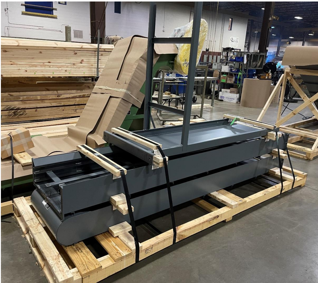
Figure 1: Example of skidded conveyor as it will be delivered to customer facility.
